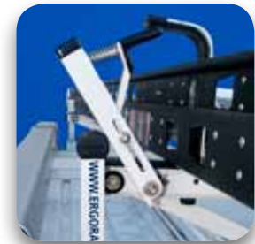
PADDED, ADJUSTABLE AUTO-CLAMP LOCKS LADDER IN PLACE WHEN STOWED TO REDUCE VIBRATION AND ENHANCE LADDER LIFE
