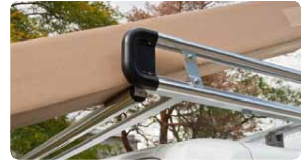
Rear Roller makes loading and unloading easy
